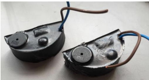
Figure 3: Prototypes encapsulated in the dielectric resin
