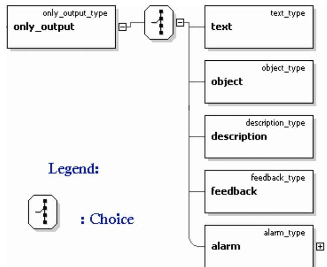
Figure 2. The specification of the *only\_output* element
