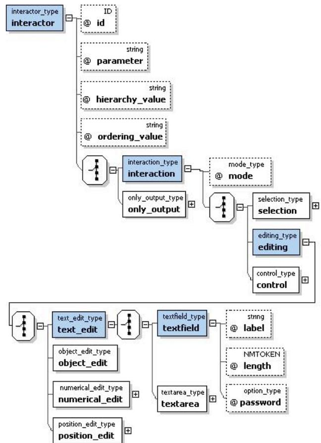
Figure 4. The specification of the *textfield* element
