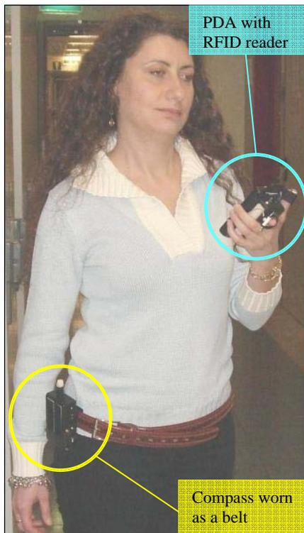
Figure 5. A blind carrying the mobile guide in the left hand and the orientation/distance detector as a belt.
