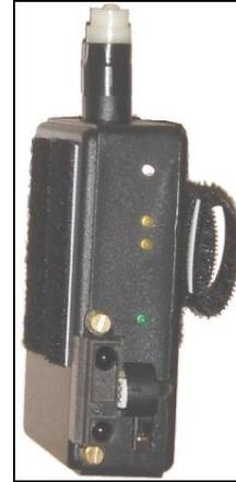
Figure 6. Detail of the compass device. The white cylinder on the top is the compass sensor; the distance sensor is located on the bottom-left.
