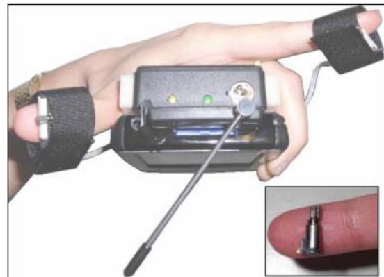
**Figure 2. iPAQ handheld equipped with the tactile module and a one of the vibrating motors adopted by the prototype (bottom-right).**
