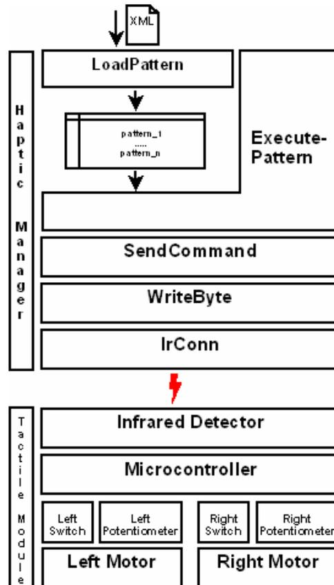
Figure 4. Hardware and software layers for the haptic framework.
