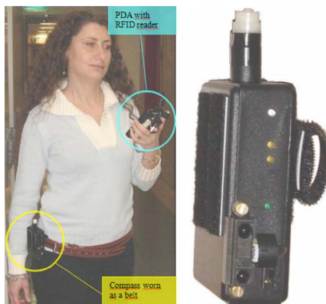
Fig. 6. Left: a blind carrying the mobile guide in the left hand and the orientation/distance detector as a belt. Right: detail of the compass device. The white cylinder on the top is the compass sensor; the distance sensor is located on the bottom-left.
